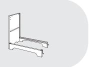
• Align side panel 2 with the dowels on base panels 3 and 4. Use one (1) A screw to fasten side panel 2 to base panel 3.
