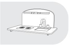
• Align the counter assembly to the rest of the kitchen assembly and fasten it in place using four (4) B screws.
