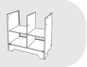
• Align back panel 8 into the grooves on side panels 1 and 2.
