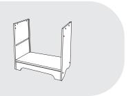
• Fasten side panel 2 to base panel 4 with one (1) A screw making sure that the dowel is aligned.
