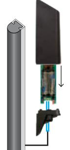
Remove Wi Edge Tx circuit board by sliding it out of housing (remove board by gently pulling down the jumper cable on the connector)
