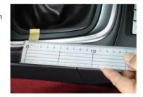
1.2 On the lower section of the passenger side center console side panel, measure 9.5cm (3.74 in.) from the seam where the center console side panel joins the center console box. Apply another piece of masking tape to mark the location.
