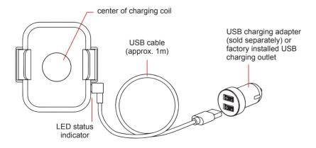
For best charging performance, place the center of the phone over the center of the charging coil
