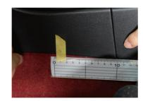
1.3 Apply the clear protective film strips to the plastic trim forward of the masking tape position markers, as shown in the illustration on the right, then remove the masking tape markers
