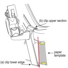
2.3 Apply medium pressure to the side of the stand for at least 20 seconds to ensure strong adhesion of the double-sided tape In cold weather, use a hair dryer to warm the mating surfaces.
