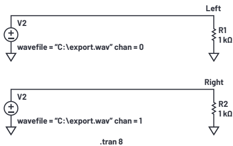
Figure 2. The two stereo channels from export.wav are used to stimulate two independent circuits.
