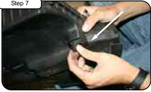
Remove the 3 rubber grommets from the air box. (To be used in step 9.)
