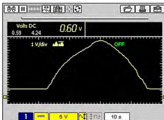
Figure C-4 Sample of Noise Filter on—TPS Sweep (KOEO)
