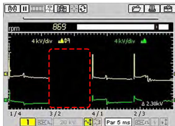
Figure D-7 Sample sensitivity set too high
