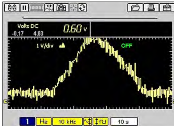
Figure C-3 Sample Noise Filter off—TPS Sweep (KOEO)
