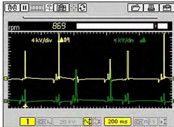
Figure D-10 Sample raw waveform of coil not firing
