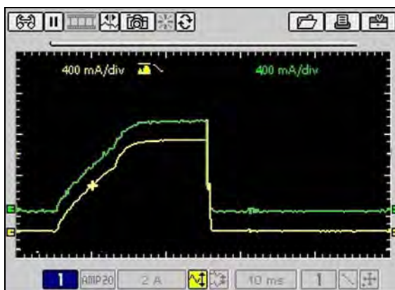
Figure C-7 Sample Noise Filter—two low amp scope probes
