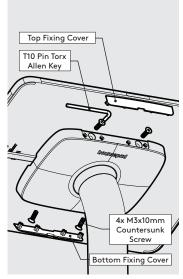
Secure the Tablet to the 10 Shell & attach the Fixing Covers as shown.
