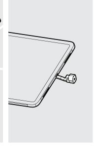
Attach the Flat Cable to the Tablet with the U-Bend Head.
