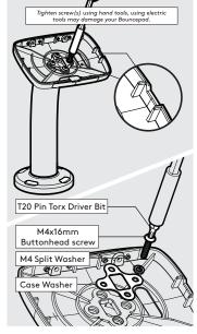
Locate & attach the Shell **B4** 5 Go to step 5. to the Static60 in the correct orientation.
