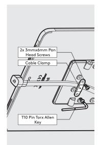
Secure the Flat Cable to the Mounting Plate with the Cable Clamp as shown.
