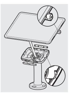
Remove the Fixing Covers. Feed the Flat Cable into the assembly & locate the Tablet in the chosen orientation.
