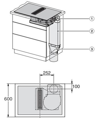
KMDA 7633, KMDA 7634, KMDA 7476 - built-in version 11 (Installation drawing)
