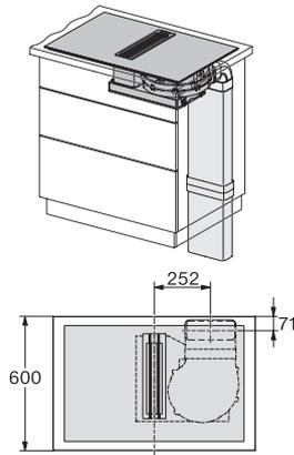
KMDA 7633, KMDA 7634, KMDA 7476 - built-in version 10 (Installation drawing)
