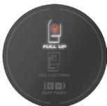
When the dust bag is full, the "FULL UP" sign is keeping high brightness, and app notice is given. Please replace the dust bag in time.
