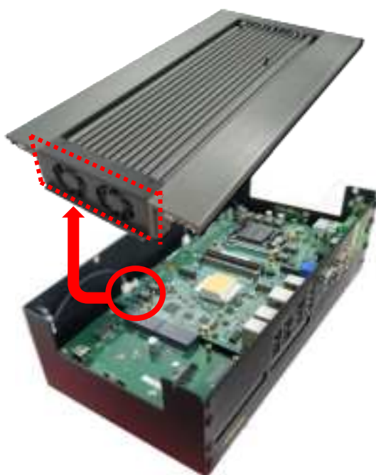
POWER1 (FAN OUT Control)
