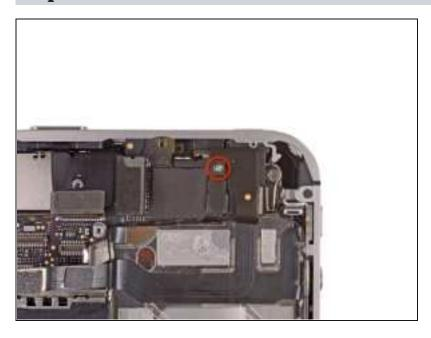
Remove the 1.5 mm Phillips screw securing the grounding clip to the logic board near the headphone jack.
