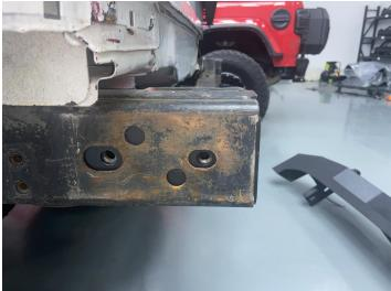
Step 4: Lift up the bumper into the vehicle frame. Install the bumper with the M12\*35 hex bolts. Tighten up those bolts.
