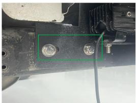
Step 5: After that put the connecting frame bracket into the rear frame gap, and than install the M12\*110 hex bolt and nuts.
