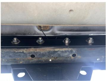
Step 6: Install the D-ring into the D-ring mount.
