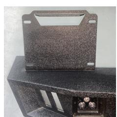
Step 3: Put the Nut Plate Brackets into the vehicle. Repeat the same procedure on the other side.
