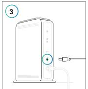
Plug the Gateway power cord into the back of the device.
