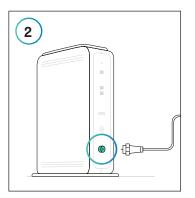
Connect the open end of your coaxial cable to the back of the new Gateway.
