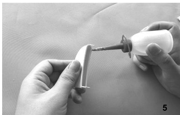
Fig. 5 - Glue the servo fairing.
