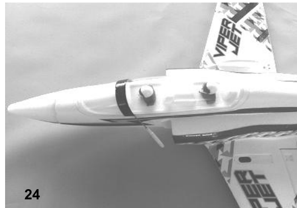
Fig. 24 - Place the fully charged flight battery in the fuselage and connect it to the electronic speed controller (Be sure the transmitter is "ON" first). The canopy is held in place by magnets and can be lifted off.
