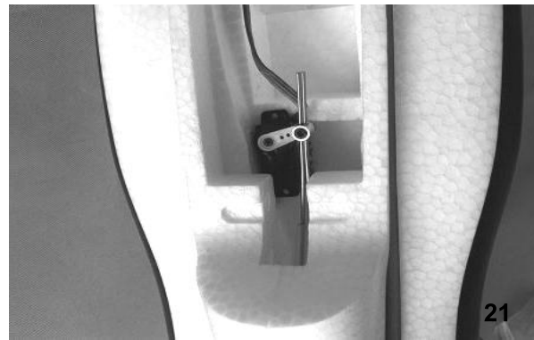
Fig. 21 - Connect the elevator push rods to the arm of servo.
