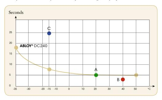
Changes in temperature have only a minimal effect on the performance of **ABLOY**® door closers and adjusted features. **ABLOY**® door closer exceeds standards demands for temperature area.
