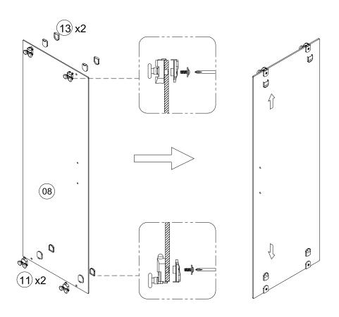
Step A: Locate the rollers into the top and bottom rails.
