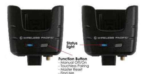
Hold while powering up for programming (LED glows solid RED)
