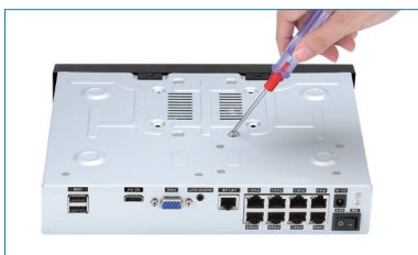
③ Screw HDD to the bottom
