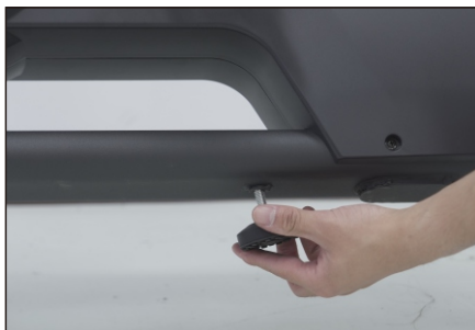
57. Tilt the machine, screw the 11# foot pad into the main frame, and then lay the machine flat. Adjust the foot pads to be leveled with the ground.
