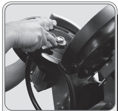
Hold wheel while loosening bolts.
