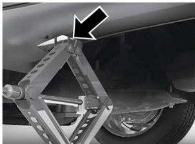
Front Jacking Location
