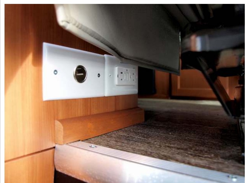
Ground fault circuit outlet behind 2nd row captains seat
