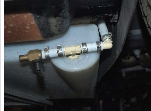
Drain for freshwater tank, beneath passenger doorstep
