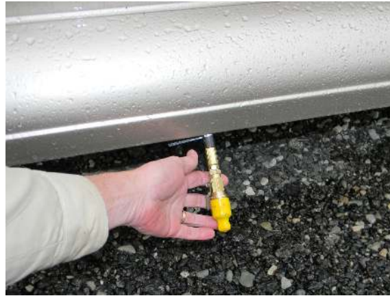
Propane pigtail, removed from retaining enclosure
