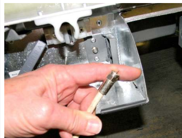
Coaxial TV connecting wire with screw-on end
