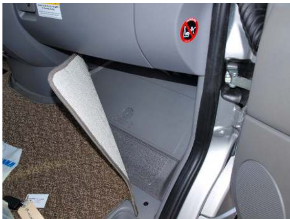
Tool access in front passenger footwell. Use a coin to turn the retaining clip and access the compartment.
