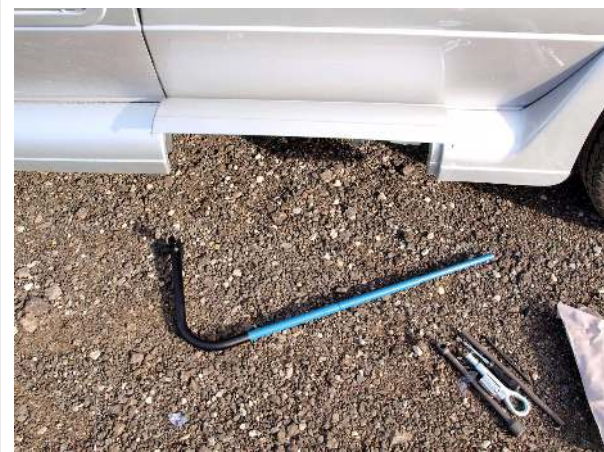
Assembled lever to lower spare tire carrier
