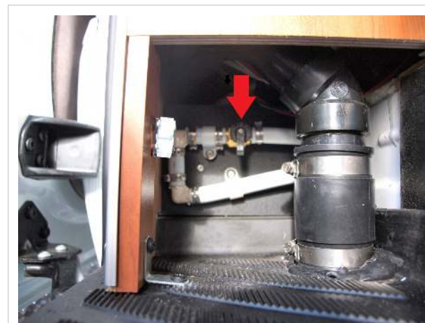
City water connection valve, shown closed
