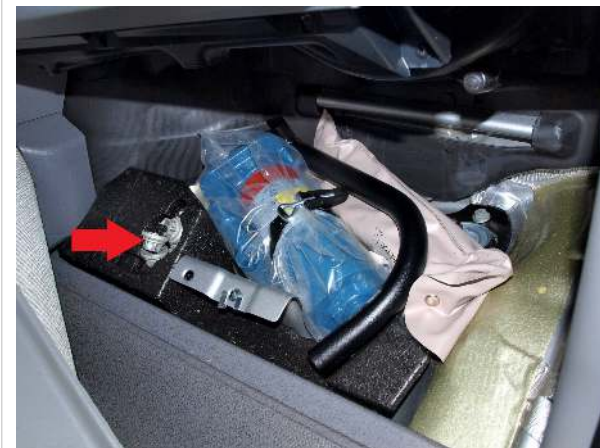
Jack, handle, and "banana" lever to lower spare tire carrier. Red arrow points to special lug nuts which MUST be used on steel spare wheel.
