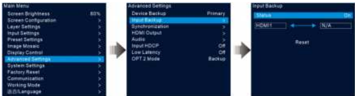
Figure 5-31 Input source backup
