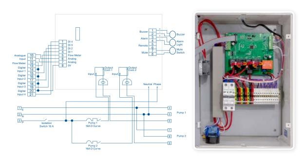
Ensure all floats are connected as normally open (NO) and as an open circuit when the float is in the down position
