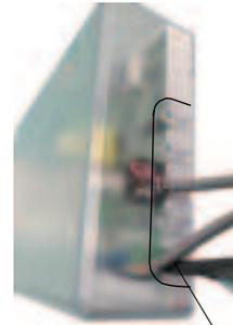
Cut off the appropriate part according to the position for wires outlet. If it is a single wire, you can cut a single wire hole, if there are multiple wires, you can cut off the cover along the maximum outline.
