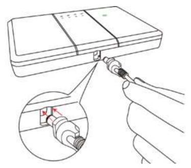
Step 2 Push the plug into place, and make a quarter turn clockwise to lock the plug.
