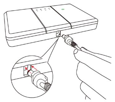
Step 2 Push the plug into place, and make a quarter turn clockwise to lock the plug.
