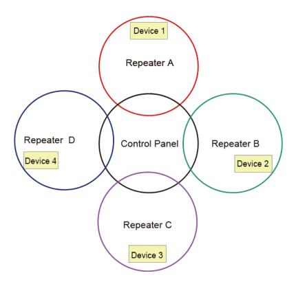
In the Example 2 below, where the Device is located between the RF coverage areas of two Repeaters, please choose **one Repeater only** to learn the Device to prevent signal traffic. **Do Not** learn a device into more than one repeater.
