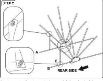
Attach supports (E) onto the side frames (A) & (B), using the fixings provided.
