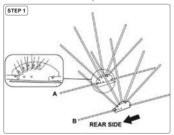
Position side frames (A) & (B) on the ground with the shortest tubes facing the front.
