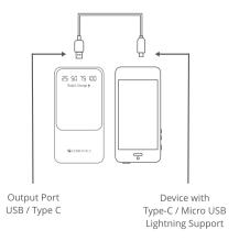
• Connect your device with the Type C connector or Micro USB or Lightning connector end of the cable and connect the other end of the cable to the power bank output port.
