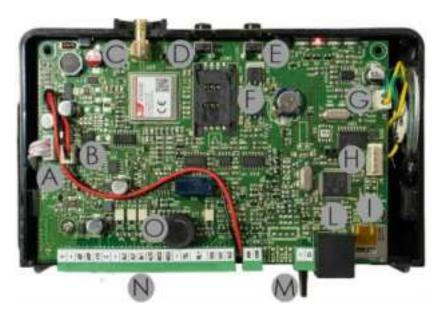
Internal power-supply connector Α В Built-in backup battery connector С Antenna cable connector D Reset pushbutton Ε Alarm pushbutton F SIM Card slot with front panel G Built-in loudspeaker connector Н Serial port for PC connection Ī MicroSD Card slot RJ11 connector for local telephone ı М Battery compartment door
