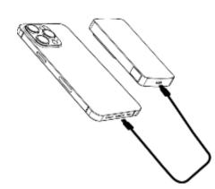
IMPORTANT: Before using your power bank for the first time make sure it is fully charged (LED displays 100%). Connect the supplied USB-C cable (or the cable that came with your device) to the power bank's USB-C port and to your device. Then begin charging your device.
