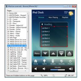
Note: Two-way lists are programmed differently on iOS devices compared to native RTI controllers. This is due to the fact that RTiPanel is exposing some of the native capabilities of the iOS scrolling lists. There is no need to account for a progress bar, or Scroll/Page up or down commands on iOS devices. The progress indicator is built into the iOS list, and swiping allows for quick, intuitive navigation through the contents of the list.
