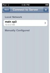
Once a server has been selected, it will provide a list of devices compatible with the hardware running the RTiPanel app. If the RTiPanel is running on an iPhone4 device, the list will show both iPhone and iPhone4 devices.
