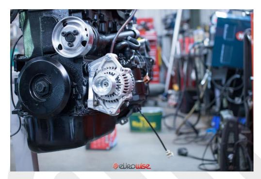
Hardware mounting locations are as following in the photos. Depending on which VR6 block you are mounting to you may not need to use all the hardware. The shortest bolt will be installed in the hole with the aluminum spacer insert installed. That one is used on 24v and 3.6 blocks.
