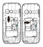
**Insert a memory card:** In order to use media player functions, a micro-SD memory card is required (not included in the package). The card must be placed into the SIM1 slot on the left
