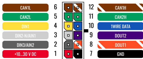
FMC250 QJIBO pinout
