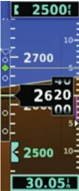
Figure 2-24 Vertical Deviation Indicator (Glideslope ILS Source) - PFD
