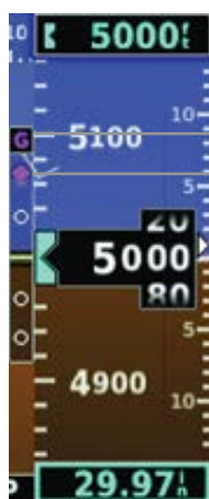
Figure 2-26 Vertical Deviation Indicator (Glidepath GPS Source) - PFD
