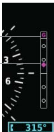
Figure 2-27 Vertical Deviation Indicator Position - HSI
