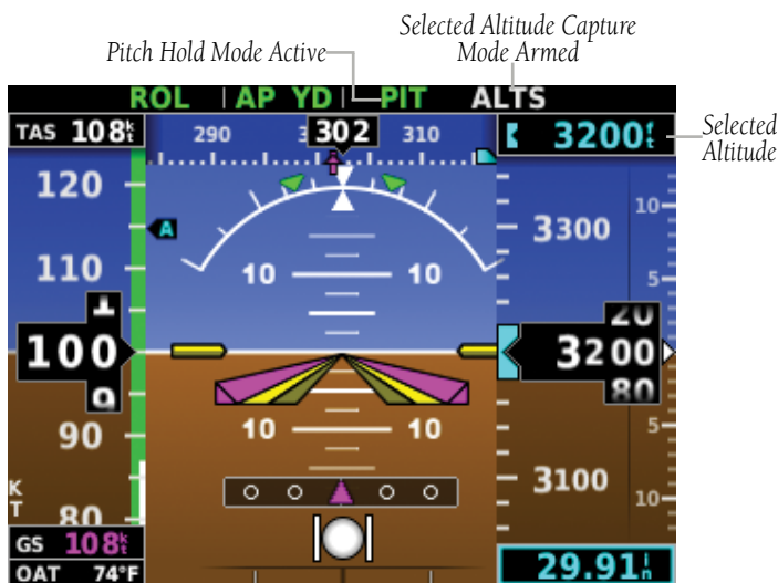
Figure 3-8 Pitch Hold & Selected Altitude Capture Modes
