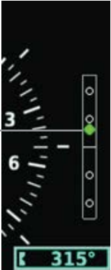
Figure 2-25 Vertical Deviation Indicator (Glideslope ILS Source) - HSI
