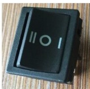
“I” – inverter is On
