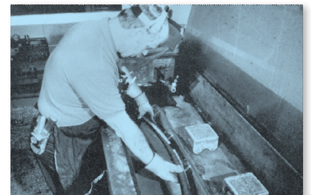
Hydrostatic hose testing.
