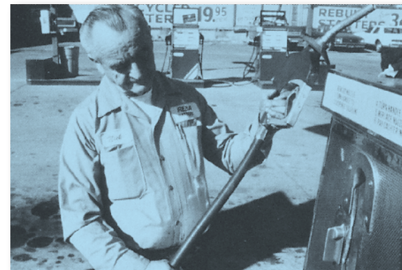
Inspect hose cover for cracks or cuts.
