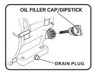
(b) Reinstall the drain plug and fill the engine with oil until it reaches the HIGH(H) level on the oil filler dipstick.
