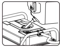
3. Install fuel cap and let any spilled fuel evaporate before starting engine.
