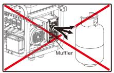
The LPG cylinder and components can be temporarily warmed by pouring warm water over them.
