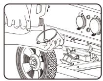
5.Replace oil fill cap/dipstick and fully tighten.
