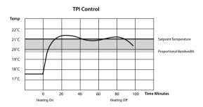
Example: Program 1 on the thermostat is  $21^{\circ}$ C for 06:30am and the room temperature is  $18^{\circ}$ C. The thermostat will start the heating at 06:30am and the room temperature will start to increase then but will switch itself off before it reaches temperature and allow the room temperature to increase naturally – this cycle may begin again if the thermostat isn't reaching temperature.
