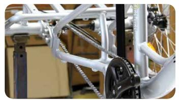
After joining the chain, mount it on the rear sprocket by carefully threading the chain onto the sprocket by turning the pedal crank arms. When the chain is secure on both sprockets, you will notice that there is excessive slack in the chain system. If ridden like this, the chain will keep falling off.
