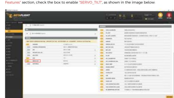
3.In the Betaflight program, select the "Servos" option from the menu bar. If the remote control channel A7 is set to a rotary switch, check the box for "Servo 1" and enable the "A7" remote control
