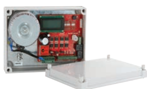
Intelligent control box with Eclipse operating system
