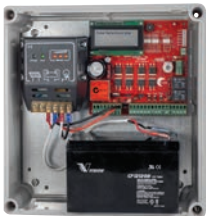
Control box with intelligent voltage doubler
