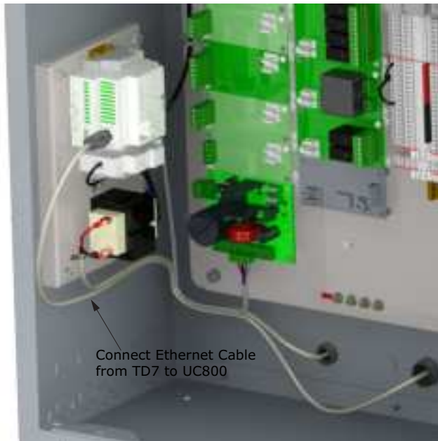
Figure 25. TD7 communication connection
