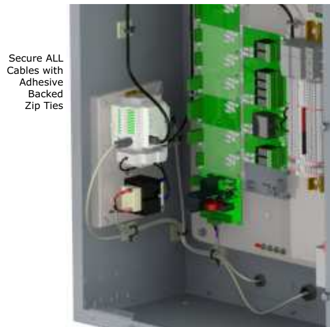
Figure 27. Secure all cables
