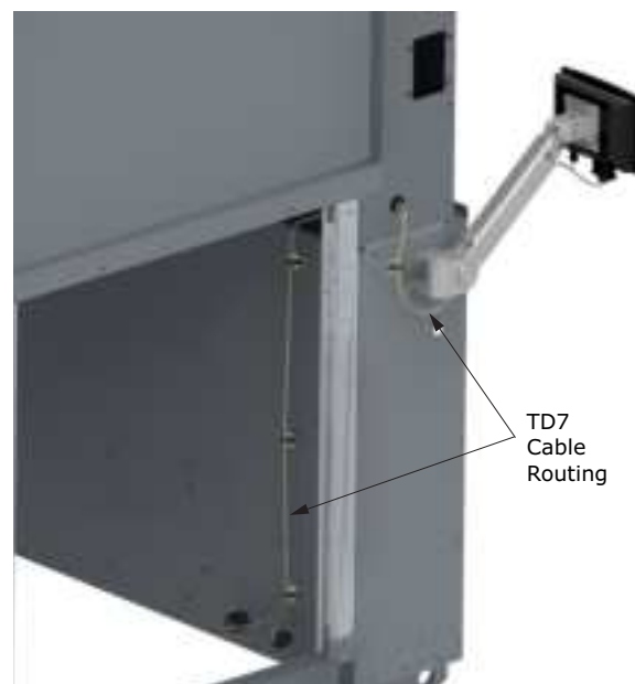
Figure 19. TD7 cable routing
