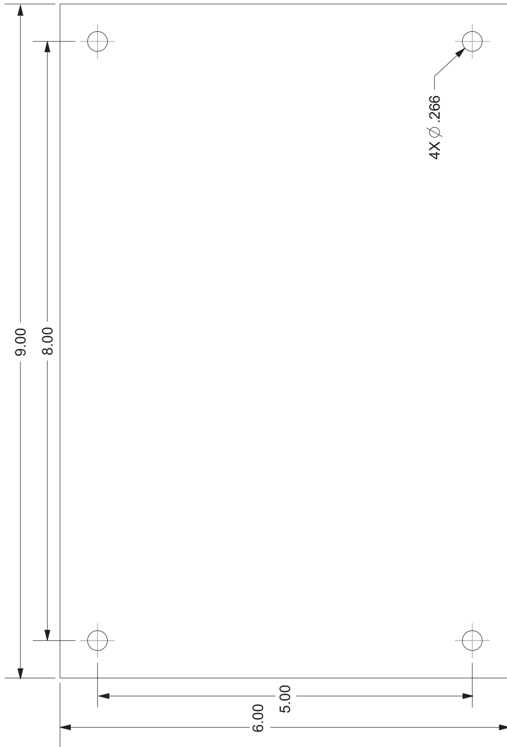
Figure 56. Back plate template (in) — actual size
