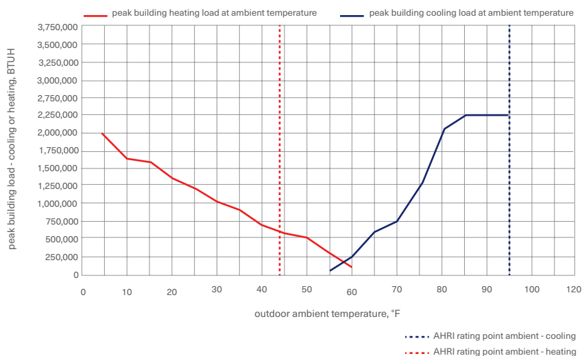
Figure 12. Peak building loads versus ambient temperature
