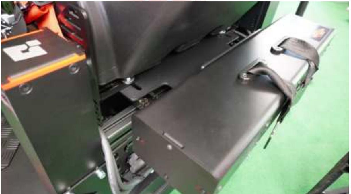
The F2MBT1 adapter is now fully installed and you can continue with the BT1 installation according to the original manual.
