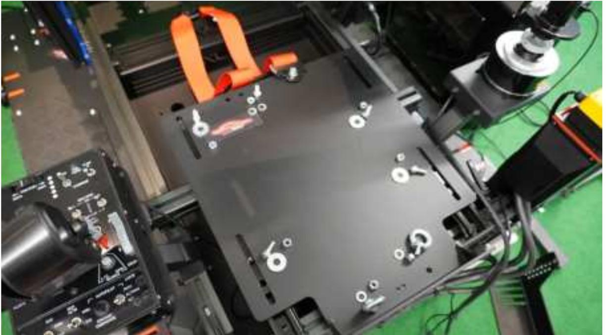
First fit the screws at the front or rear. To do this, carefully move the seat slider forwards or backwards to reach the screw head. Caution: risk of injury! Use 4x M8x20 hexagon socket head bolts, each with a large washer and an M8 lock nut. When fitting a seat from the side, screw the seat angle loosely (!).
