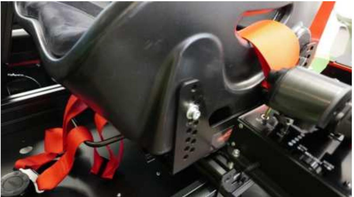
Now tighten all screws (after tight comes off!). Now check the smooth running of the seat slider directly. If it is blocked or very stiff, something has been installed at an angle or tilted!
