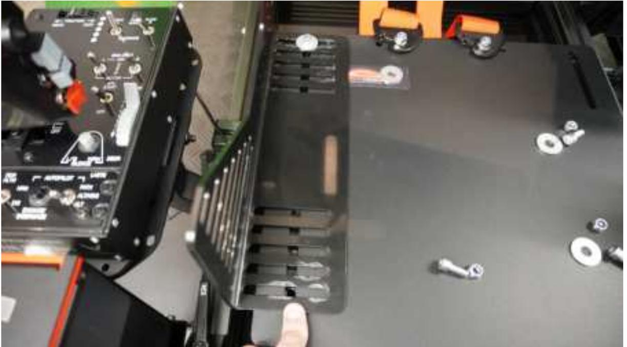
Now measure the required seat inside width and align the seat brackets. Then screw on the other side (front or rear). Again, adjust the seat slider as required. Do not tighten these screws either.
