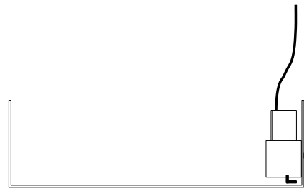
Deep drip tray side mounted using bracket (Sensor not to touch a conductive drip tray)
