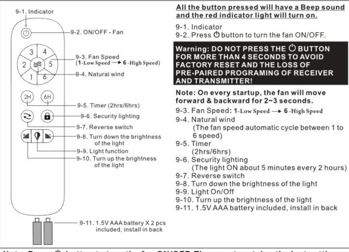
Note: Press (b) button to turn the fan ON/OFF. The remote retains the last settings (fan speed and light dimming level) in memory. Switch the fan ON/OFF by main power will operate at initial setting. (fan off and light on)
