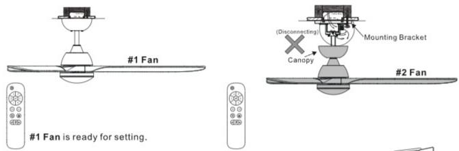
Turn on power at breaker box and #1 Fan is ready for pairing.
