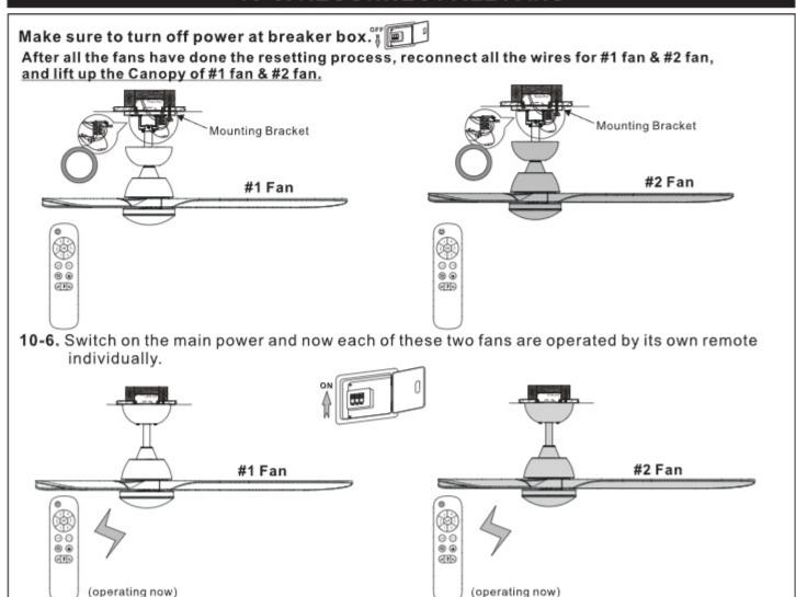
**NOTE:** For more than two fans, the same rules apply. Make sure only one fan at a time is connected to power when doing the Remote Setting. Already completed fans should be disconnected until all fans have completed the Remote Setting process.
