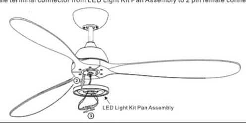
A Rotate the Light Kit Pan slightly until two pre-installed screw heads are engaged in the narrow end of key holes.
