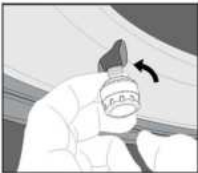
c. Screw the anti-theft nut counterclockwise against the sensor wrench
