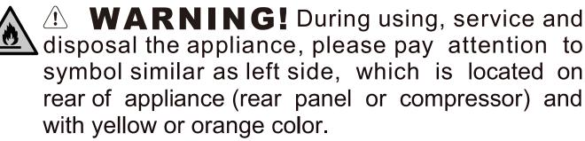
fire warning symbol. There risk of flammable materials in refrigerant pipes and compressor.
